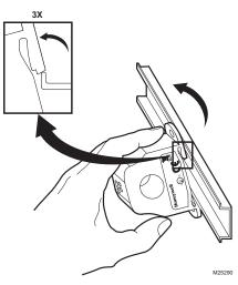
Fig. 2. Sensor removed from DIN rail
